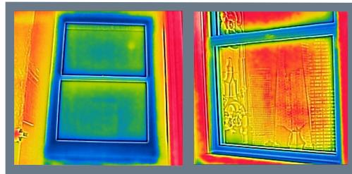
In these thermal images — cooler temperatures are shown in blue, while warmer temperatures are shown in red. On average, the surface temperatures of the new windows are 9 degrees Fahrenheit warmer in the winter than the old windows.
