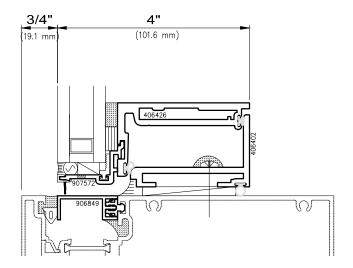
Read-through of glazing components may be evident from the exterior using certain glass types.
