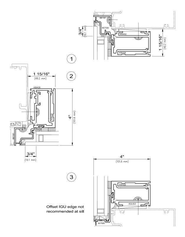
Read-through of glazing components may be evident from the exterior using certain glass types.
