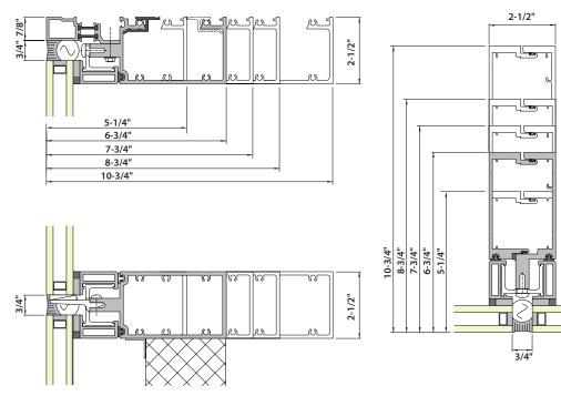
Designer Note: The use of clear glass in four-side silicone-glazed wall systems can make insulating glass unit construction, as well as glazing materials, visible under certain exterior lighting conditions. Review samples carefully during glass selection.
