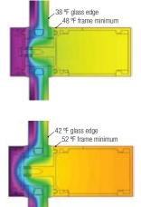
SuperWall with aluminum pressure plates
