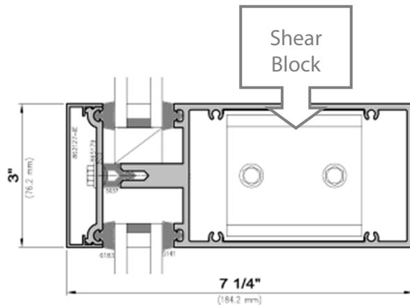
“Stick wall” systems are shipped in pieces for **field-fabrication and/or -assembly**. These systems can be furnished by the manufacturer as “stock lengths” to be cut, machined, assembled, and sealed in the field, or as “knocked down” parts pre-machined in the factory, for field-assembly and -sealing only.
