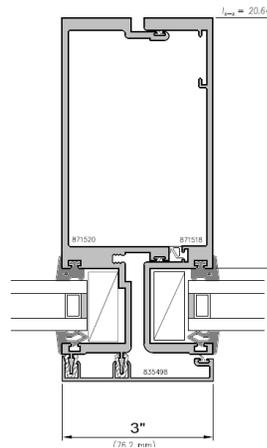
Factory-assembled and factory-glazed under controlled conditions
