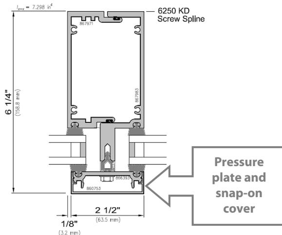
Some stick curtainwall is called “**pressure wall,**” because exterior extruded aluminum plates are screw-applied to compress glass between interior and exterior bedding gaskets. A snap-on cover or “beauty cap” is then used to conceal fasteners.
