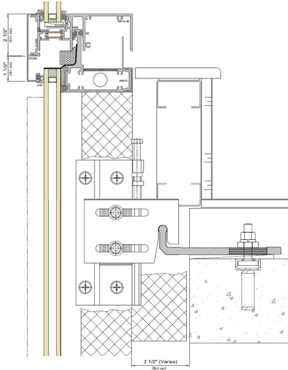
In some applications, the curtainwall dead load weight is transferred to the base of the wall, through vertical mullions.
