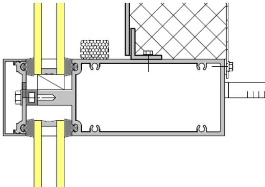
Incorporating shadow boxes can lend spandrel areas a degree of depth and transparency. However, under certain transient weather conditions, internal condensation may form.
