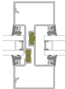
“**Storefront**” is a non-load-bearing glazed system that occurs on the ground floor, which typically includes **commercial aluminum entrances**. It is installed between floor slabs, or between a floor slab and the building structure above.
